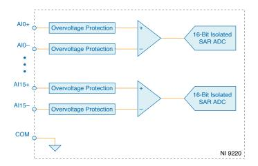
• Input signals on each channel are buffered, conditioned, and then sampled by an ADC.
