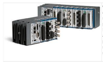
CompactRIO combines an open-embedded architecture with small size, extreme ruggedness, and C Series modules in a platform powered by the NI LabVIEW reconfigurable I/O (RIO) architecture. Each system contains an FPGA for custom timing, triggering, and processing with a wide array of available modular I/O to meet any embedded application requirement.
