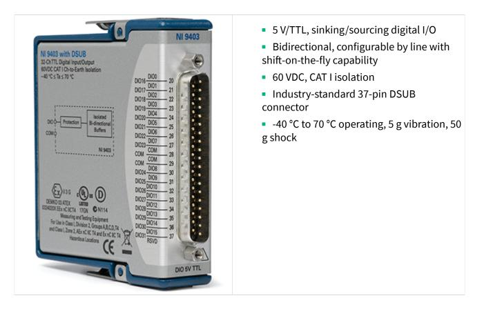
The NI-9403 is a 32-channel, 7 μs bidirectional digital I/O module for any NI CompactDAQ or CompactRIO chassis. You can configure the direction of each digital line on the NI-9403 for input or output. Each channel is compatible with 5 V/TTL signals and features 60 VDC, CAT I isolation. The NI-9403 also features ±30 V overvoltage protection and can source up to 2 mA output current per channel.
