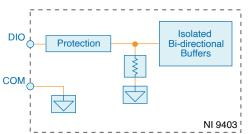
The DIO channels have Schmitt trigger inputs and are compatible with 5 V/TTL logic devices. Each input channel has hysteresis for improved performance with noisy and non-monotonic input signals. Each channel also has a pull-down resistor.
